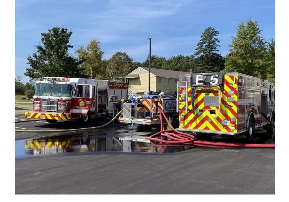
September 26, 2023. Consistent with the SFD vision of "always ready, constantly improving, and ever vigilant", the City's apparatus undergo annual pump testing to ensure the safety, operational capability, and reliability of the fire pumps which are rated from 1500 gallons per minute to 2000 gallons per minute.
