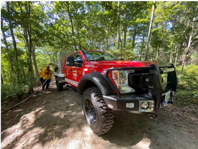
September 17 SFD personnel with assistance from Dover Fire and Rescue operate at a brush/wildland fire in the Willand Pond recreational area. Pictured here is “the beast” – the unofficial nickname for the SFD forestry unit – with twin reel (“booster”) lines in operation operating off tank water along a narrow trail.
